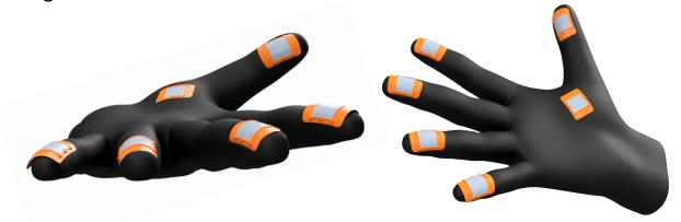
This means the PAF-1419 can convey specific material textures and familiar sensations to users more naturally than other devices. Specific waveforms can be designed to convey impacts of any type – such as the click of a button or dice rolling across a table – or more complex haptic stimulus, like feeling water ripple across the hand.
