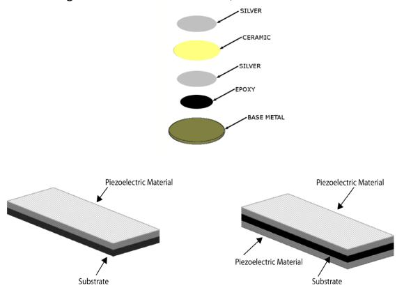
Based on the reverse piezoelectric effect, these actuators consist of layers of active piezoelectric ceramic that bend and contract outward when voltage is applied. Attaching this piezoelectric material to a base metal or a substrate causes an out-of-plane displacement when voltage is applied. This physical displacement generates the haptic feedback experienced by the user- the extent of which is directly influenced by the capacitance of the piezoelectric system.
