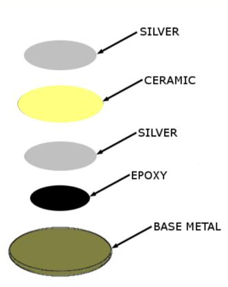
A lead zirconate titanate (PZT) crystal is coated with silver on both sides, glued to a brass, nickel alloy, or stainless-steel disk.
