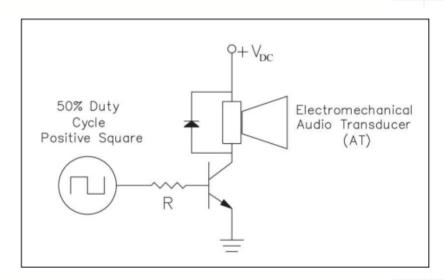
The positive transducer terminal connects directly to the voltage rail, which needs to be within the transducer's operating voltage range. Input to the base of the transistor should of high enough voltage from the processor, to ensure that the transistor is driven hard to the ground to allow the transducer to oscillate at the input frequency.
